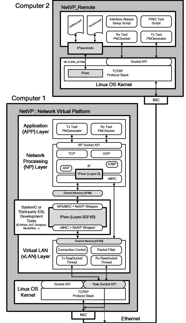
Figure 2. System architecture of the NetVP
