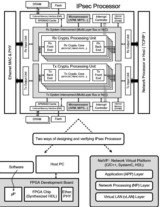
Figure 1. Design and verification methods of IPsec Processors
