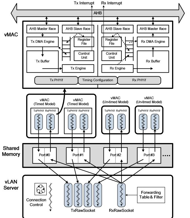
Figure 3. The architecture of the vLAN and vMAC
