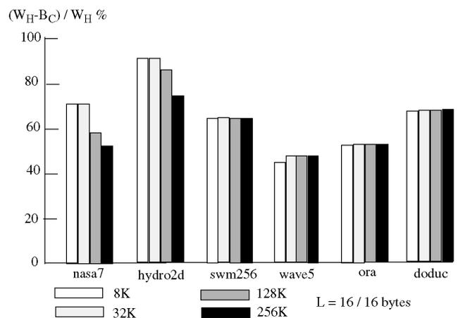
Fig. 6. Saving of write-hit memory cycles using the RFDB protocol ( $L = 16$  bytes).
