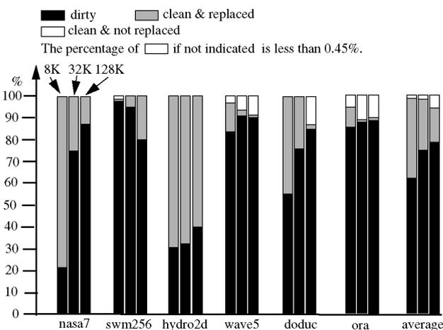
Fig. 8. Cache line usage for the SPEC programs ( $L = 16$  bytes, write allocate cache, set-associativity = 2).
