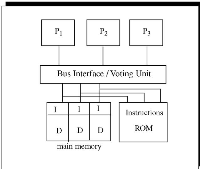
Fig. 1. A triplex fault-tolerant computer system.
