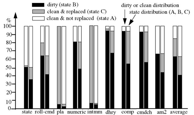
Fig. 10. Cache line usage for the flight control programs (L = 4 bytes, write allocate cache, set-associativity = 2).
