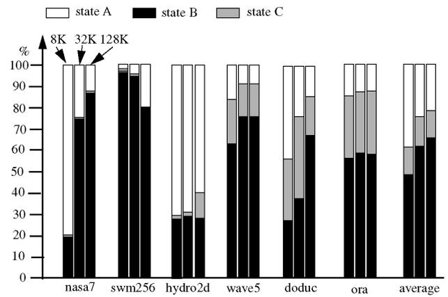
Fig. 9. Cache line state distribution ( $L = 16$  bytes, write allocate cache, set-associativity = 2).
