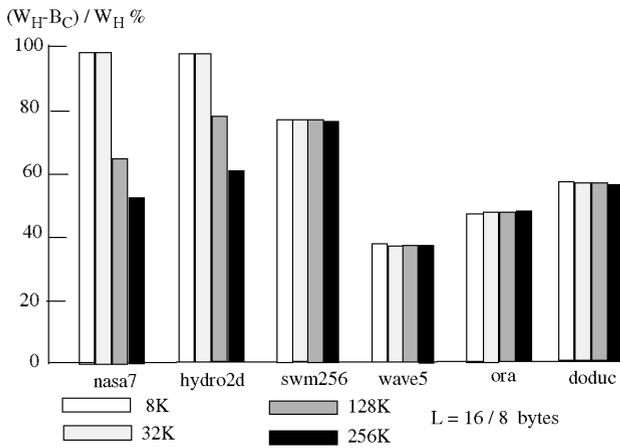
Fig. 7. Saving of write-hit memory cycles using the RFDB protocol ( $L = 16$  bytes, subblock size = 8 bytes).
