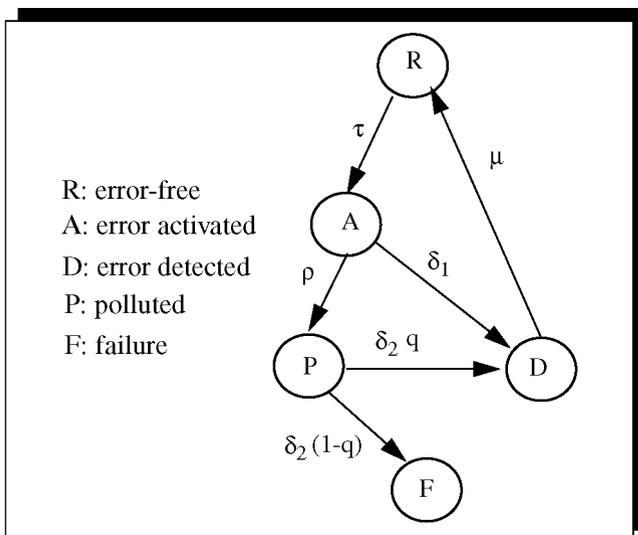
Fig. 2. A cache error model for transient faults.
