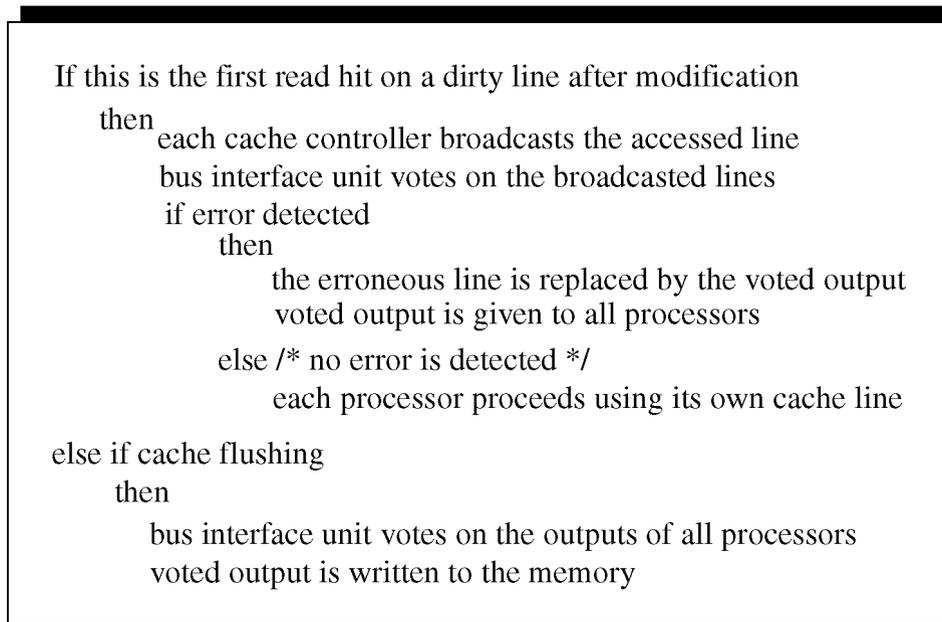
Fig. 3. The Read-First-Dirty-Broadcasting protocol for write-back caches.
