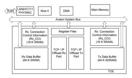
The interconnection of these components was configured using the SOPC Builder tool, and the data was transferred into each component through Avalon system bus. Our TOE features the following five external channels:
