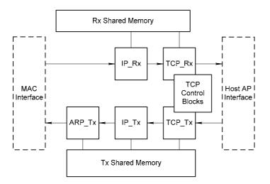
Figure 5. Protocol Processing Module Required for TCP Packet Processing & Shared Memory
