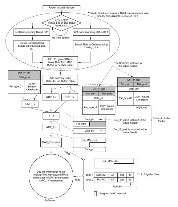
Figure 12. Process Flow of Transmitting Packet
