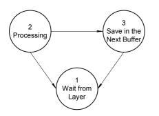
Figure 7. State Machine Structure of Protocol Processing Module
