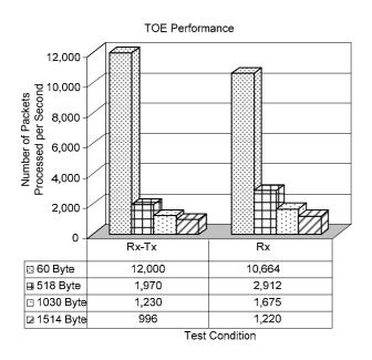
In Rx-Tx testing, when the packet size is 60 bytes, the number of packets processed by the TOE per second can go up to 1514 bytes (packet size). This is because the TOE has three data replications from receiving to transmitting: the first from MAC buffer to TOE RxBuffer, the second from TOE RxBuffer to TOE TxBuffer, and the third from TOE TxBuffer to MAC.
