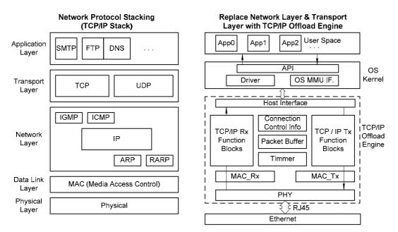
Figure 1. Network Protocol Stacking (TCP/IP Stack) & TOE Engine
