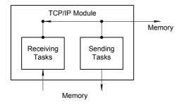
Figure 5 shows the relationship between the TCP packet processing module and the buffer. After the protocol processing is finished on the first layer, the processed data is discarded to the next layer in order to avoid too much memory-to-memory transfer, so that the processing module of each communication protocol will be able to read and write using a shared memory.
