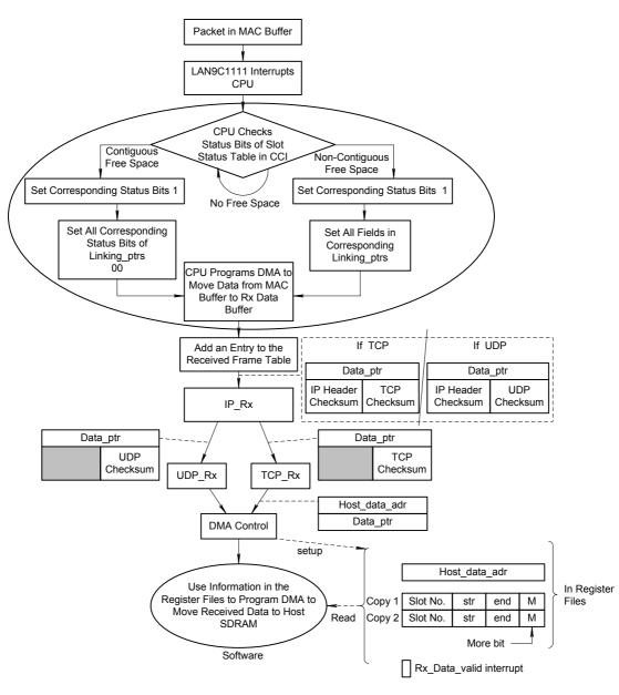
Figure 13. Process Flow of Receiving Packet
