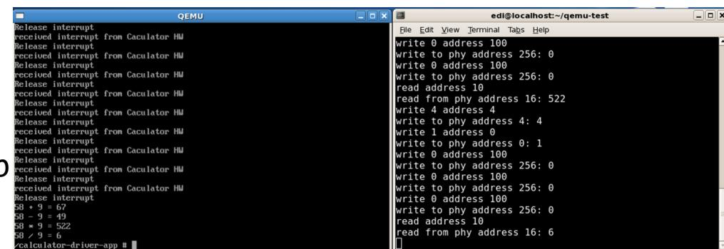
The image shows two terminal windows side-by-side. The left window, titled 'QEMU', displays a series of interrupt logs from a calculator application. The right window, titled 'edi@localhost:~/qemu-test', shows SystemC-level memory access logs, including writes and reads at specific addresses.
