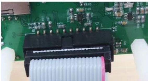
Figure 9, connecting JTAG cable
