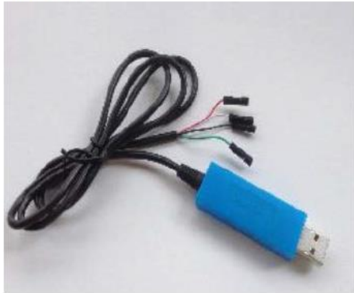
Figure 6, USB to TTL(3.3V) cable
