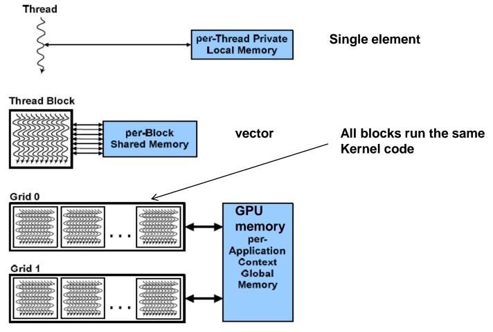
CUDA Hierarchy of threads, blocks, and grids, with corresponding per-thread private, per-block shared, and per-application global memory spaces.
